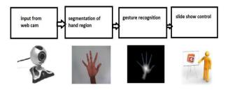
Figure1. Architecture for hand gesture recognition
